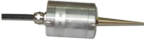
One-component velocimeter made with a special strong motion sensing element. While small in size and light, these sensors feature high level of accuracy and stability of parameters.
